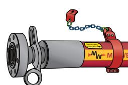
TEST HOSE CKRED-56-10K 3.5" ID 10000 PSIW.P. RED CHOKE AND KILL HOSE 1234 01/16 -4° to 212° F 15000 PSIT.P. MANUFACTURED TO API SPEC7K 1234 01/16 -20° to 100° C INSPECT HOSE FC
